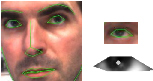
Figure 1. Left: face features detection as seen by the iCub. Right: eye area detection (top right) and extracted eye area with detected pupil center as seen by the iCub (bottom right).
