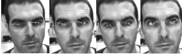
Figure 3. Gaze tracking estimates using our system.
